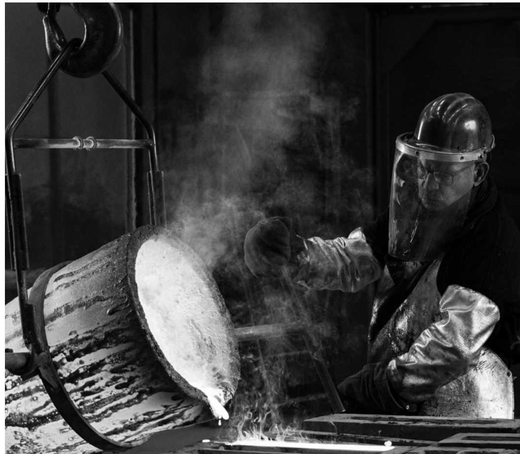
Bronze Foundry Kemner, Bronze, Sand Cast Methode, 2023 Photo: Micky Hoogendijk
